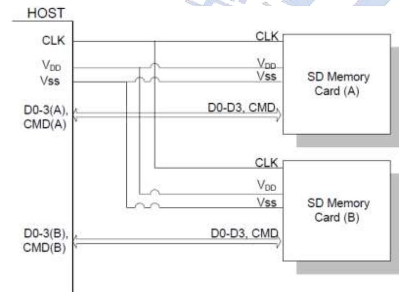
Figure 3-2 SD Memory Card System Bus Topology
