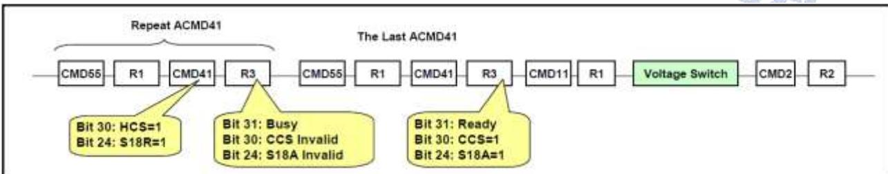
Figure 3-5 ACMD41 Timing Followed by Voltage Switch Sequence
