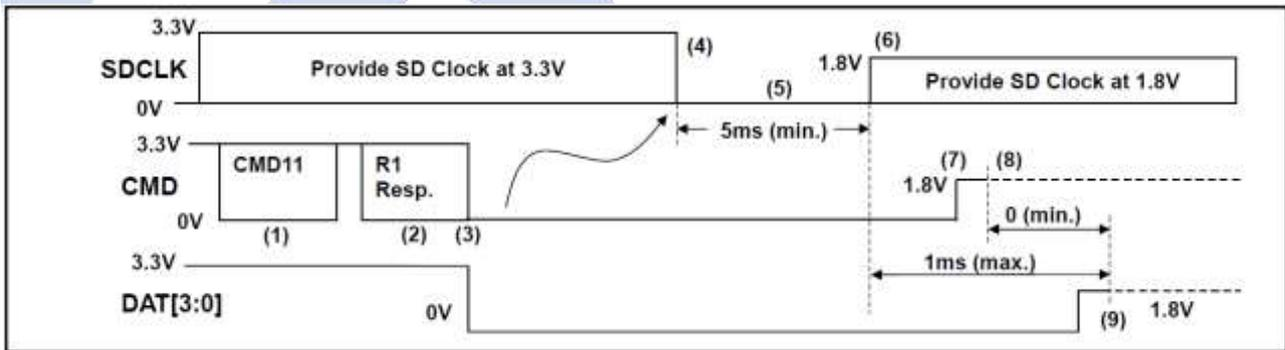
**Figure 3-6 Signal Voltage Switch Sequence**
