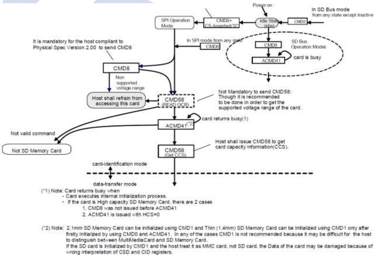
Figure 3-3 SD Memory Card State Diagram (SPI mode)
